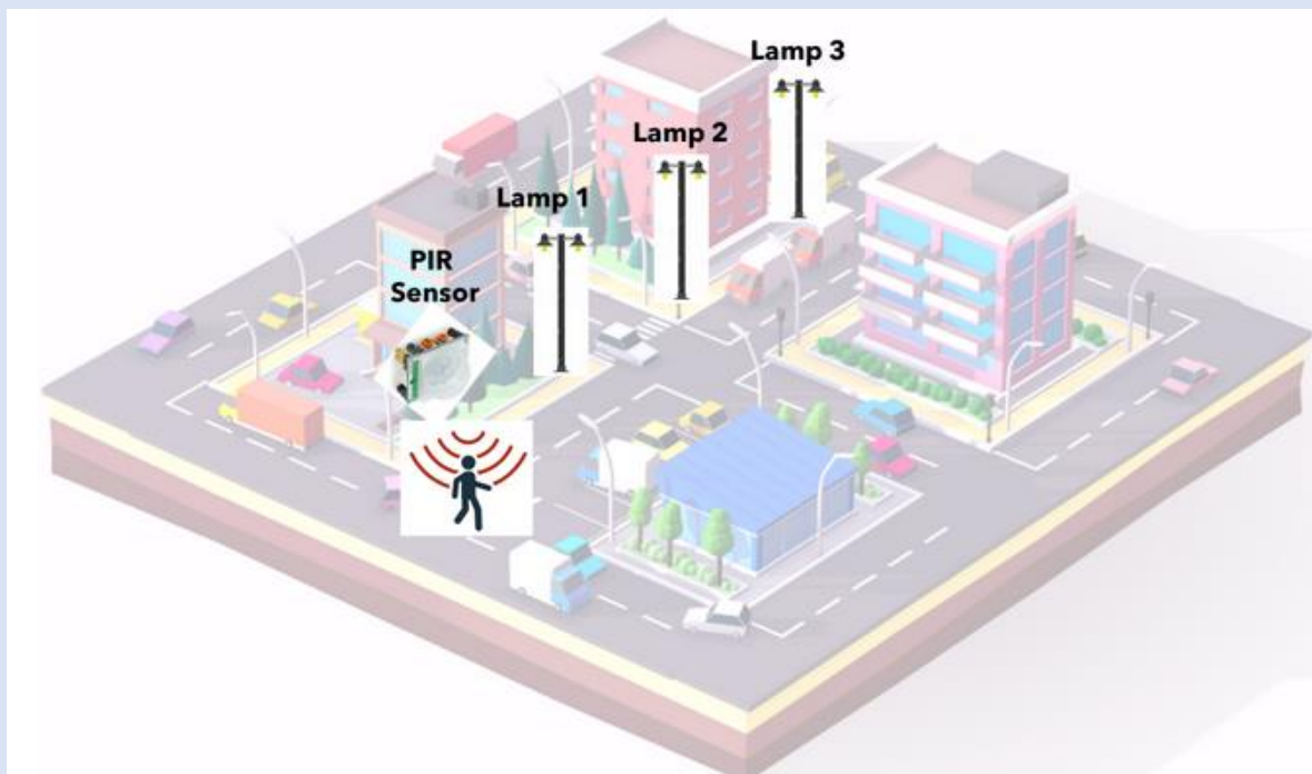
Figure 8 - A model of a street equipped with a movement sensor and LED lamps.
