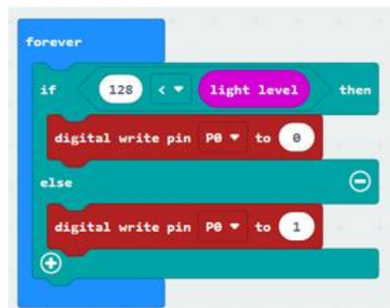
Figure 5 - An example of block coding to turn on a LED.
