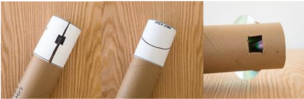
Position the CD at a 30-degree angle with the tube
